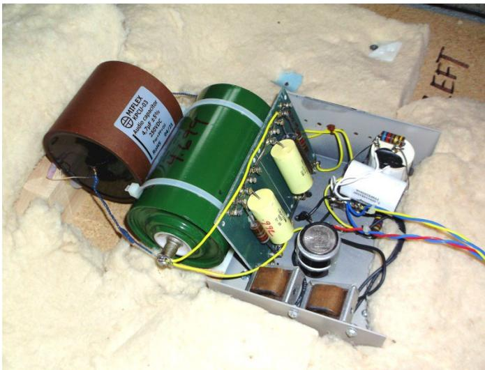
Also damping resistors, with values as low as 350-ohms across capacitors, but no higher than about 600-ohms -- and across coils that should be at least 500-ohms. These resistors prevent series/parallel capacitor/inductor resonances that can mimic mechanical colorations. The real world has me using 450-ohms in each case and they work well.
