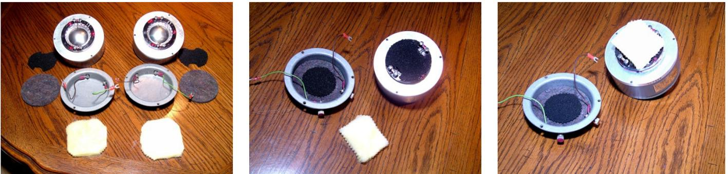
The horns themselves needed damping and I used a combination of lead sheet, ceramic tiles, clay sealants together with RTV silicone. Lead sheet and tiles adhered with silicone provided constrained layer damping. After all of the work I did there was still a metallic coloration that I thought I would have to live with.
